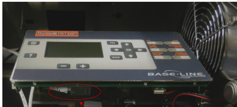
Ethernet port on the back of the FlowStation module
