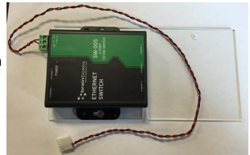
5. Locate the 2 long screws that were provided with the Ethernet switch. Working from the outside of the pedestal, push the screws through the holes on the pedestal wall and through the holes on the Ethernet switch mounting plate.
