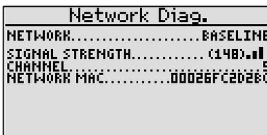
You might be able to boost the strength of your wireless signal by changing the orientation of your antenna. Watch the number in the signal strength field while you change the antenna orientation. A larger number indicates increased signal strength.
