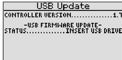
The USB Update screen displays the current firmware version at the top. If your controller is running firmware version 1.7 or lower, you will need to download a firmware update onto a USB drive from the Baseline web site, and then install it on your controller.
