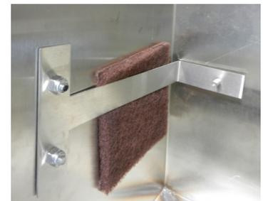
Baseline's left mounting bracket on top of the vent mesh
