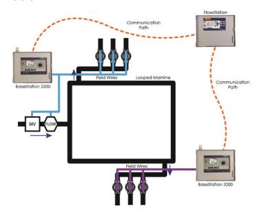
After all components in the shared flow group are communicating and configured, the BaseStation 3200 asks the FlowStation for water to run the zones in a program. The FlowStation allocates the water, and the programs start based on their priorities.
