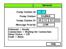
6. In the Pump Station ID field, press the + button to set the ID to a number 1 through 8.
