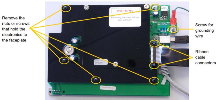
10. Gently lift the display electronics away from the back of the faceplate. Put the electronics in a safe place.
