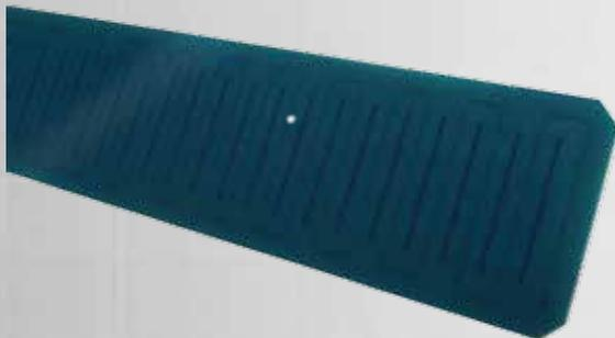
Baseline Soil Moisture Sensors work by sending a high frequency pulse of electricity down an embedded wire path. The high frequency of the pulse causes the sphere of influence to move outside the sensor blade and into the soil around it. When the pulse travels through moisture, it slows down. The sensor measures the speed, and then converts this measurement to a moisture content reading.
