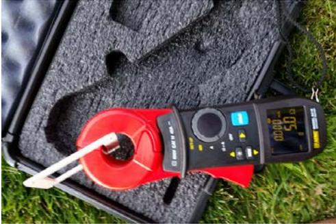
3. If you do not read 5 ohms, clean the heads of the Clamp-On Ground Tester and repeat from step 1 above.
